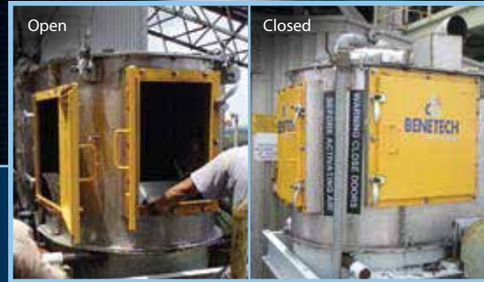
Custom head chute prevents material and dust build-up, while the innovative design allows full interior access
