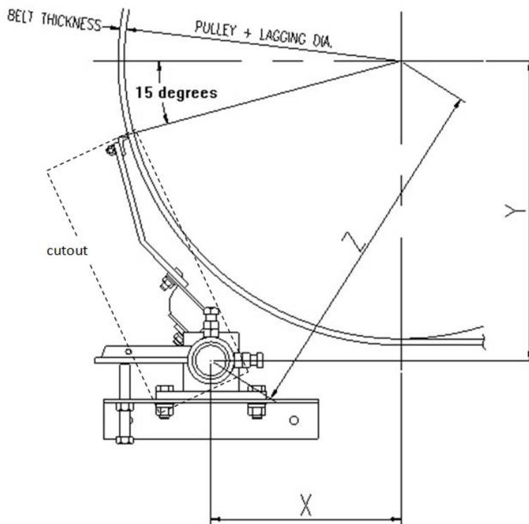
Figure 2 : Mounting Location
